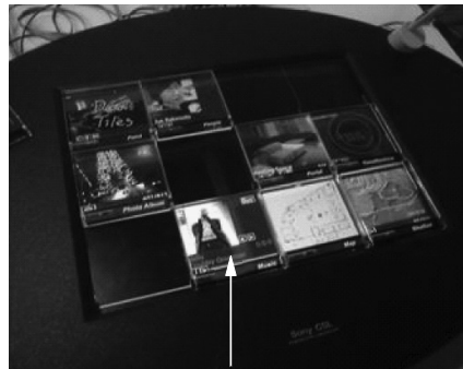
b) Construction of interactive programs by assembly of physical tablets identifiable by RFID
